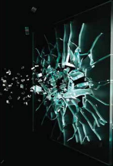
Annealed Glass Large, dangerous shards
